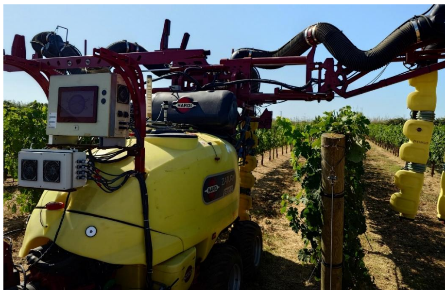
Figure 3: precision variable rate spray machine for vineyards. Capable for applying different water volumes to different zones/blocks of the vineyard following a prescription map. It has been extensively trialled on commercial vineyards, demonstrating that targeted application according to canopy density significantly reduces the quantity of PPPs required to manage the crop. It is ready to be commercialised.
