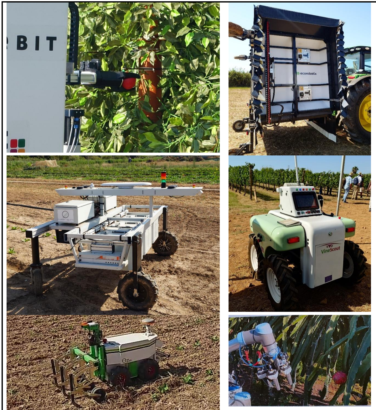
Figure 2: Top left: HARVBOT, robotic harvesting in apples (still in R&D). Top right: Ecorobotix, precision automated smart spray machine for vegetable crops (commercialised). Middle left: Earth Rover, scouting and weeding (non-pesticide) robot (commercialised). Middle right: VineScout, scouting and mapping robot for vineyards (ready to commercialise). Bottom left: Oz naio technologies, soil preparation, seeding, weeding robot (commercialised). Bottom right: scouting and harvesting robot for dragon fruit (still in R&D).
